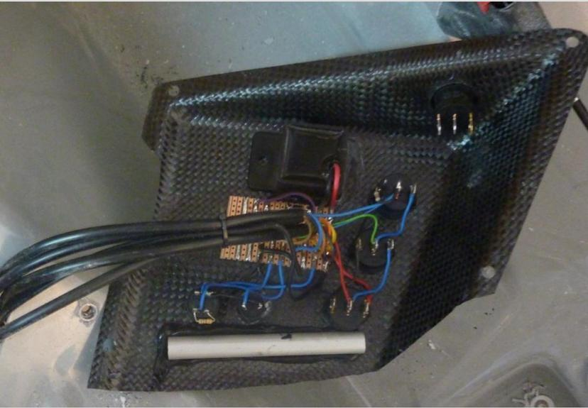
The wiring is connected to the dashboard, here showing the inside. In this case, an extra switch is installed at the side of the dashboard for the interior lighting. Install a piece of aluminum tube with some kit in order to stiffen the dashboard
