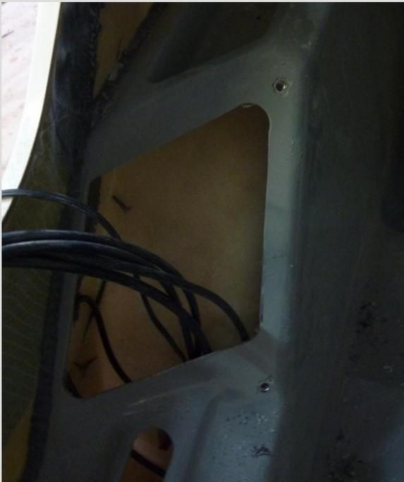
Size the dashboard to fit it on the inner shell. Hold the dashboard in place and drill two holes 5 mm at indicated locations through both the dashboard and the inner shell. Re-drill the holes in the inner shell to 7.5 mm. Push rivet insert nuts in these holes and fasten it using a rivet insert nut plier (see part 5 'covers').
