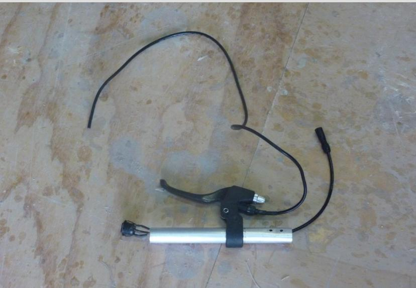
Dis-assemble the steering handle (screwing the Allen screws inwards), slide the brake lever over the steering handle and feed the electric cable through the handle. The turning signal switch on the left handle, the horn and signaling switch on the right handle. Next re-assemble the steering handles.
